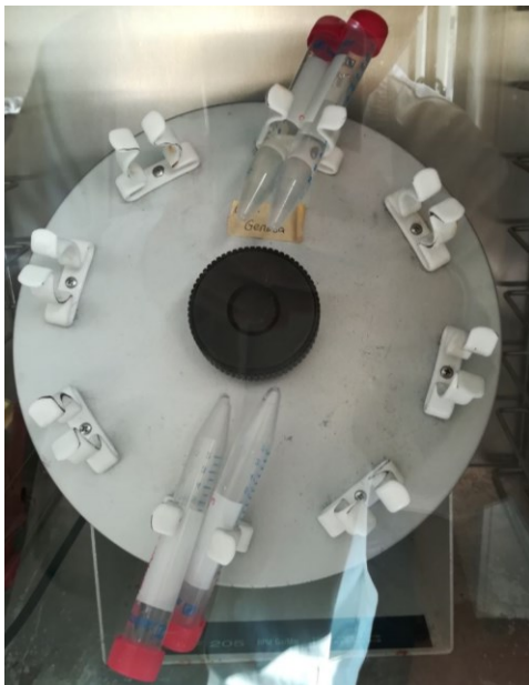
Figure 2.7 Four samples of tissue in buffer with papain placed in a rotary shaker in the oven at 60°C
