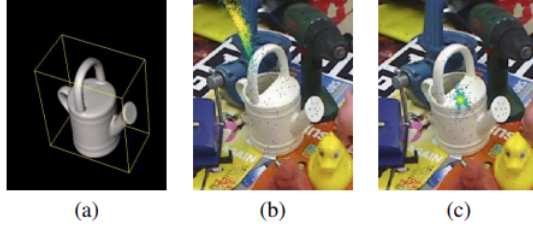
Figure 2.17: (a) A 3D object model and its 3D bounding box. (b) Hypotheses produced by PVNet for a bounding box corner. (c) Hypotheses produced by PVNet for a keypoint selected on the object surface. The smaller variance of the surface keypoint shows that it is easier to localize the surface keypoint than the bounding box corner in our approach.
