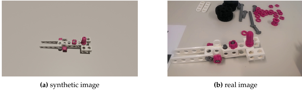
Figure 7.1: Comparison of real and synthetic images showing assembly state 11 from a similar viewpoint. The main difference is the presence of loose parts in the real image.
