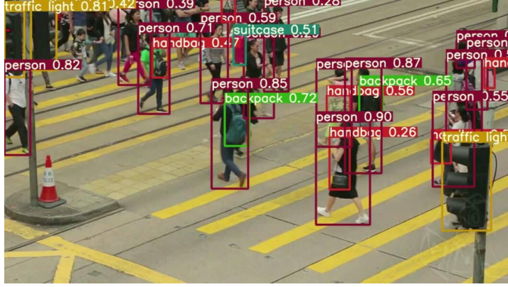
Figure 3.2: Example of object detector inference results. The model identifies relevant objects by generating bounding boxes with associated labels and each prediction is assigned an overall confidence score.
