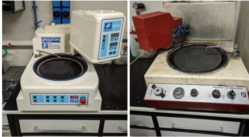
Fig. 3.7: Lapping machines used to polish and roughing the samples
