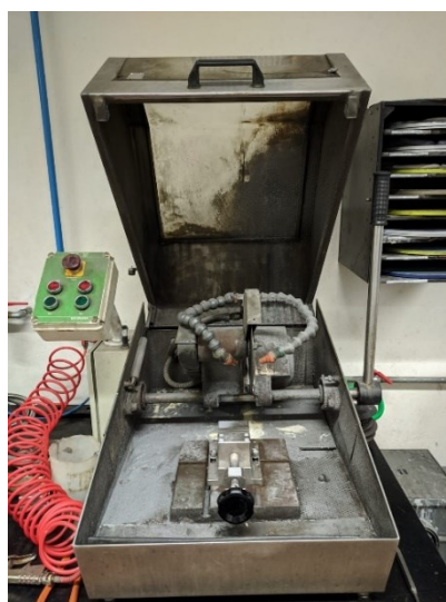
Fig. 3.6: Cutting machine used for material preparation
