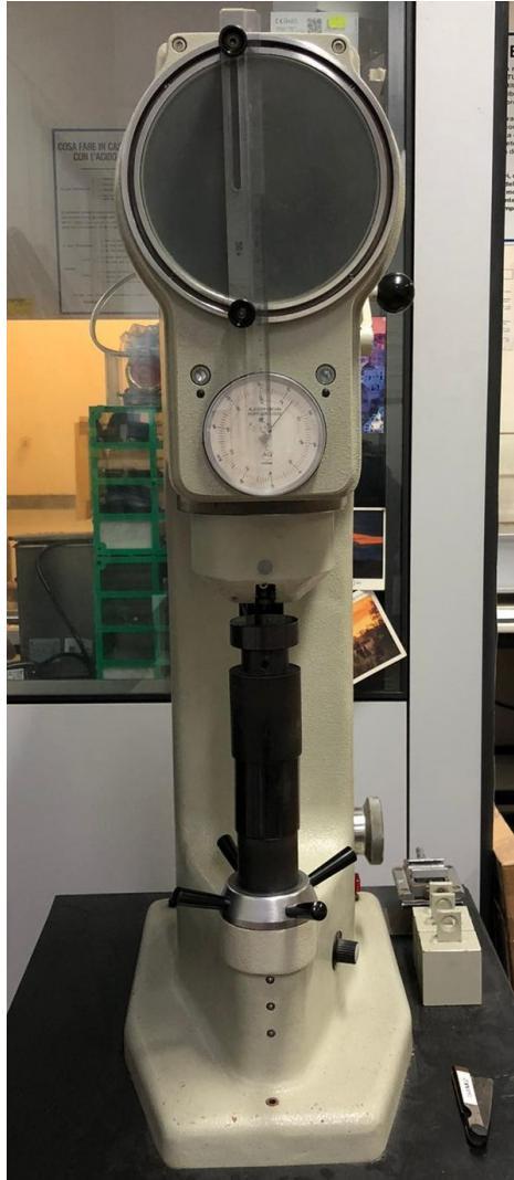
Fig 4.13: The durometer used for the hardness test
