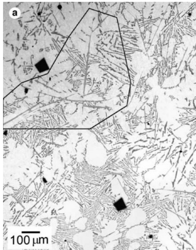
Fig. 1.7: The \beta -Fe phase has a lamellar morphology [13]
