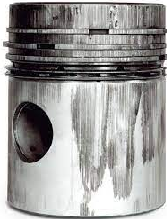
Fig. 1.5: Wear rate effects on a piston [5]
