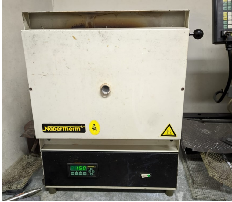
Fig. 3.3: The preheat furnace used to dehumidify the die
