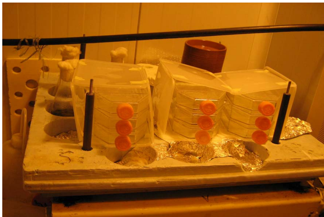
Figure 2.8: The flasks of culture with the light protection structure placed in the phytotron.
