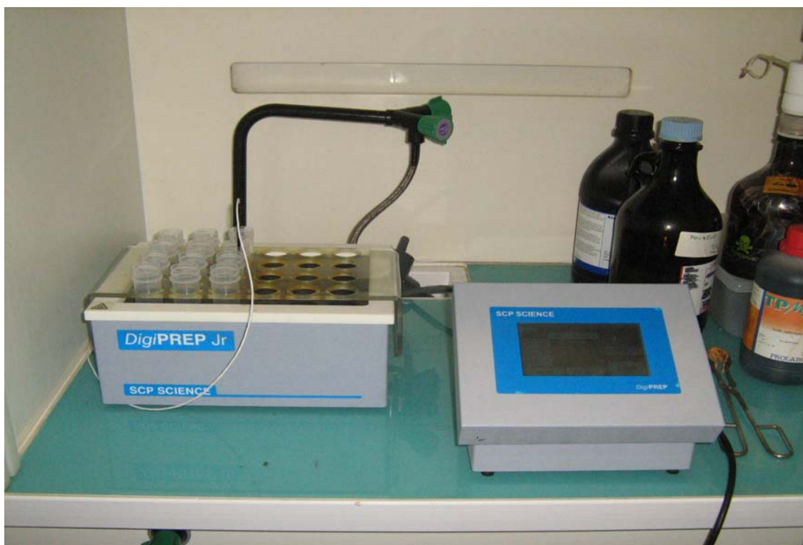
Figure 2.19: Samples of diatoms treated with H 2 O 2 30% in the digester (DigiPREP Jr., SCP SCIENCE, Canada) used to prepare the frustule identification.
