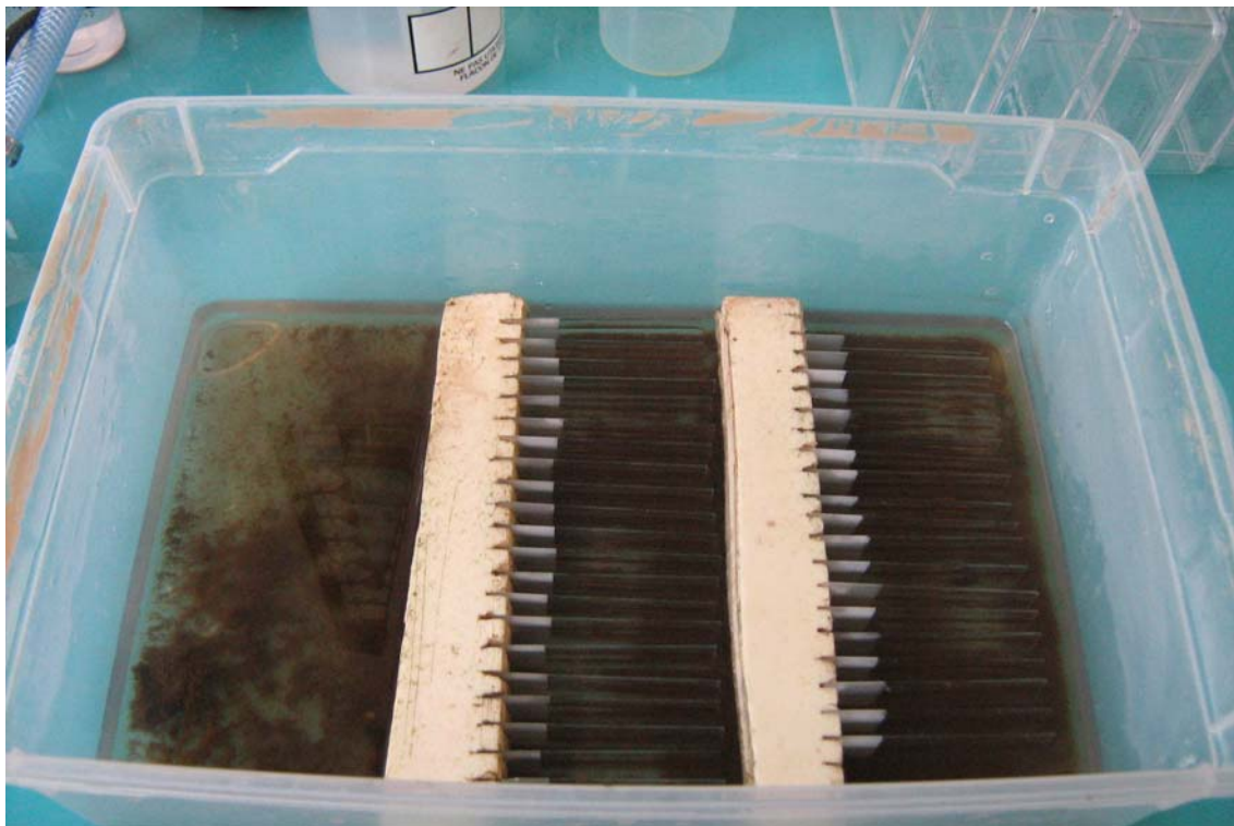
Figure 2.6: Plastic box with vertical slides to isolate benthic diatoms.
