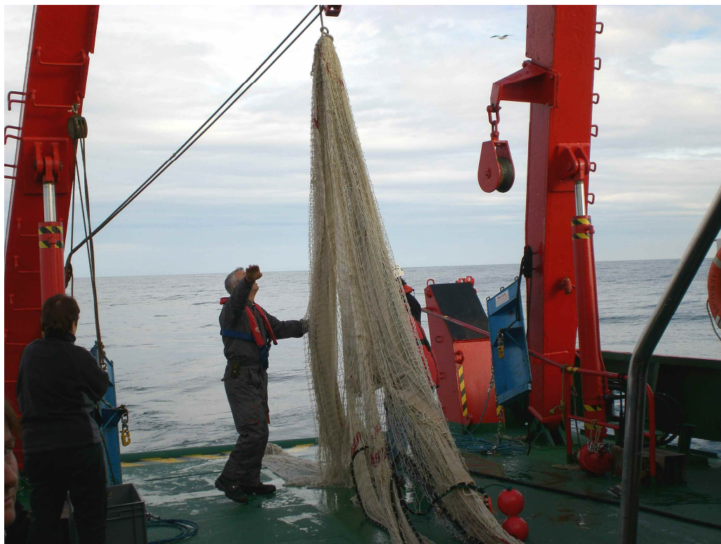
Figure 4 - Retrieving a Sardonet pelagic trawl net.
