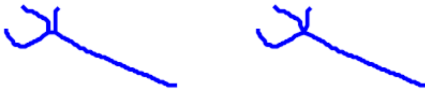
Figure 2.20: The skeleton after pruning short external branches and after eliminating short internal branches.[55]
