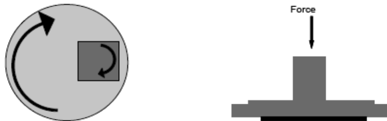
Figure 20: Drawing of the polishing equipment seen from above (left) and the sample holder seen from the side (right).
