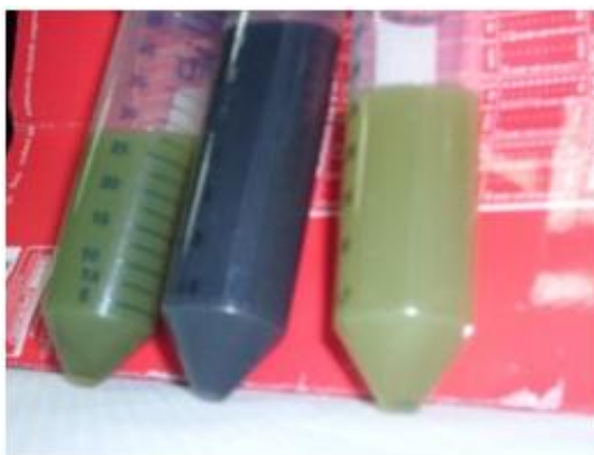
Fig. 62: CNT@diazo-SH@CdS, CNT@diazo-SH@ABQ1 and CNT@mercaptopilane@CdS just after sonication
