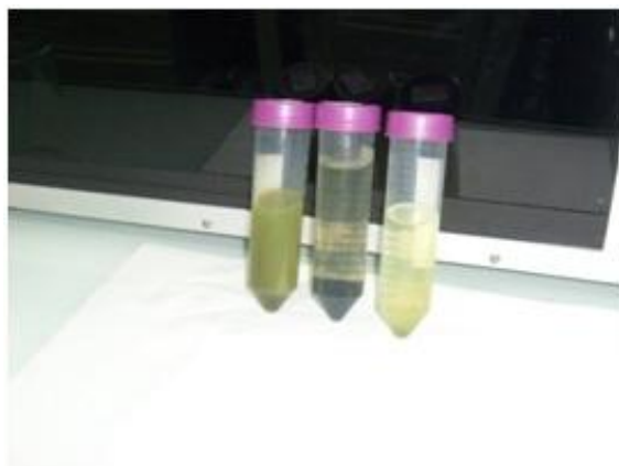
Fig. 63: CNT@diazo-SH@CdS, CNT@diazo-SH@ABQ1 and CNT@mercaptopilane@CdS after 1 sedimentation week
