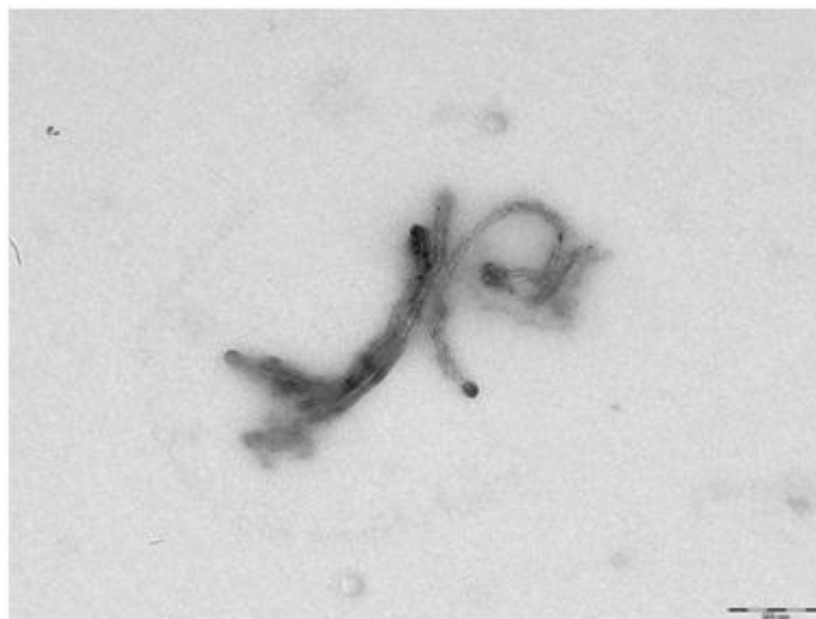
Fig. 42: CNT@mercaptosilane: oxidized CNTs functionalized with a mercaptosilane
