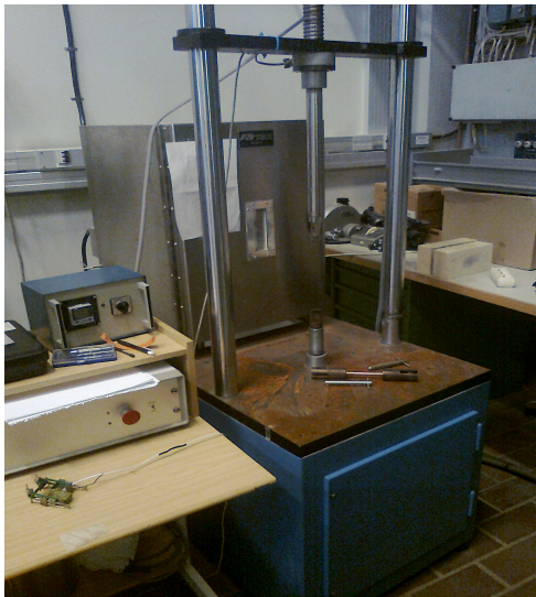
Fig. 7: Machine for tensile tests
