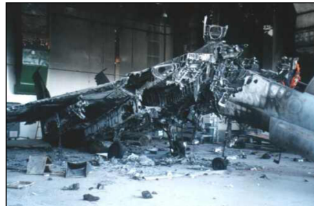
(d) F-15 destroyed by Human ESD contact caused by an improperly grounded fuel container during maintenance
