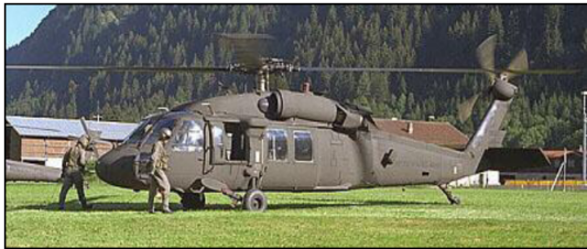
(a) UH-60 Black Hawk. Most of its crashes since 1982 were caused by flying too close to radar and radio transmitters and even citizens band (CB) transmitters, because of the susceptibility of the electronically controlled flight system to these EME
