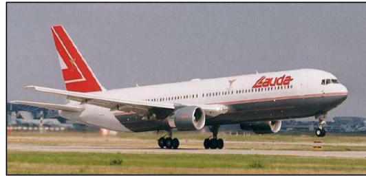
(b) On May 26 1991 the Lauda Air flight 004 crashed into a jungle shortly after taking off from Bangkok. It was supposed, that EMI from a camcorder, a laptop or a mobile phone could have turned on the left engine thrust reverser
