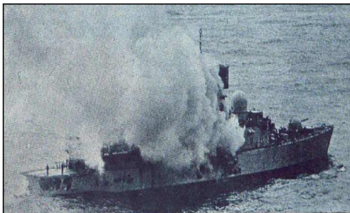
(c) On May 30 1986 the UK lost the destroyer HMS Sheffield. Because of interference between the communication radio system with the antimissile detection system, this last one was turned off during communications. Unfortunately this coincided with the enemy missile launch
