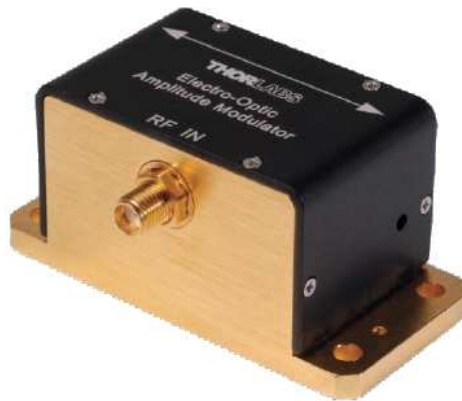
Figure 3.8: Thorlabs EO-AM-NR-C4 LiNbO_3 polarization modulator. The 2mm hole in the right-lower part of the housing is the beam entrance. An SMA input connector allows connecting an external high-voltage driver needed to operate the modulator.
