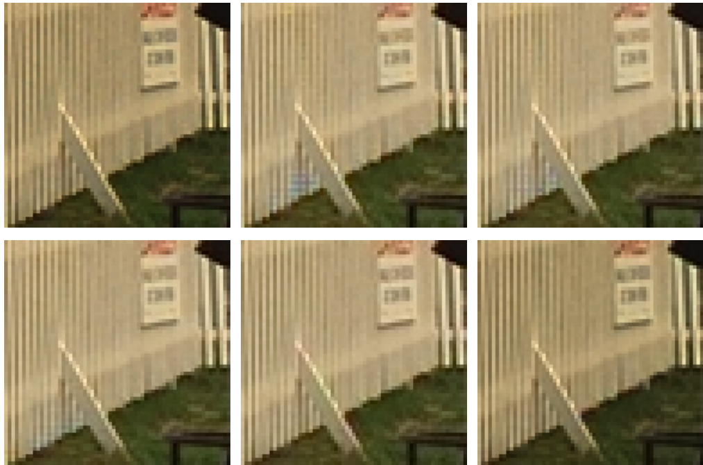
Figure 5.6: Comparing the visual quality provided by different demosaicing algorithm on a detail of Kodak image 19.
