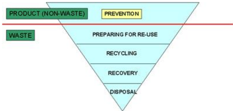
Figure 1.1 Waste management hierarchy according to the European Directive 2008/98/CE ( http://ec.europa.eu/environment/waste/framework/ )
