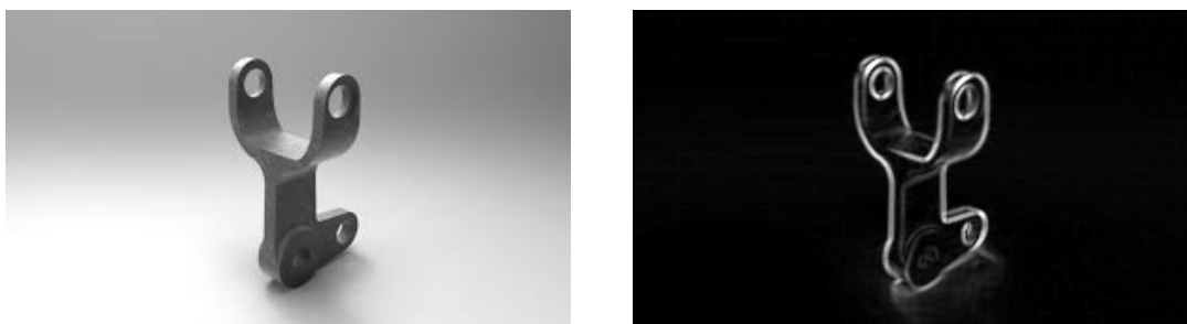
Fig. A.3: Image representing a generic component on the left and the result of Sobel operator on that image on the right.
