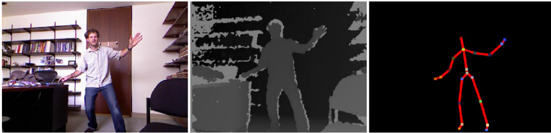
Figure 3.10: This image shows the various steps of skeleton tracking in a Microsoft Kinect sensor: on the left the scene viewed from the RGB sensor, on the center the image from the depth sensor and on the right the identified human links.
