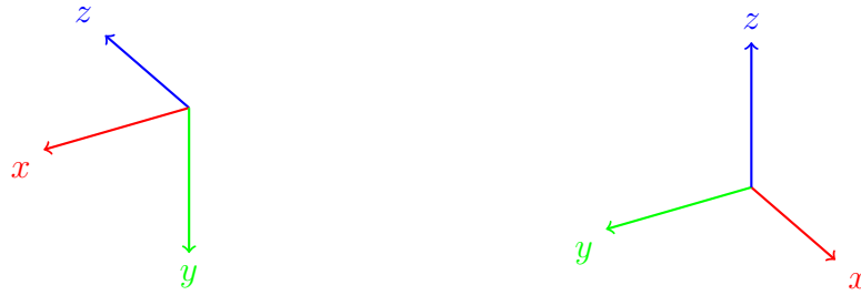
Figure 4.8: On the left the Cartesian coordinate system of the human model and on the right the coordinate system of the robot model.
