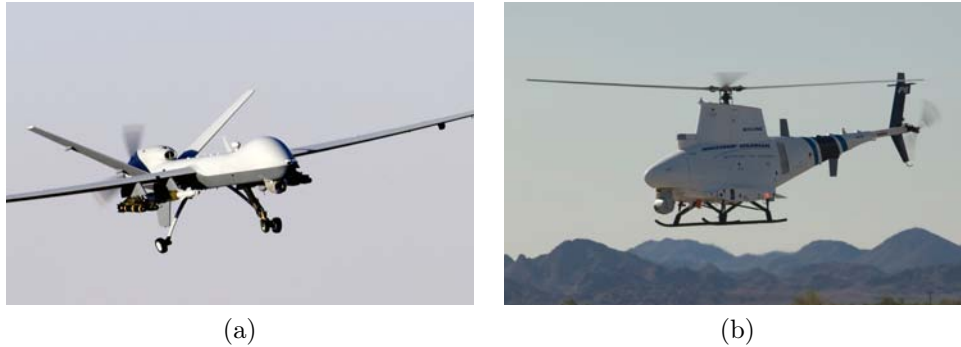
Figure 2.2: Two different types of UAVs. (a): MQ-9 Reaper is a fixed wing hunter-killer surveillance UAV. (b): MQ-8 Fire Scout is an unmanned autonomous helicopter.
