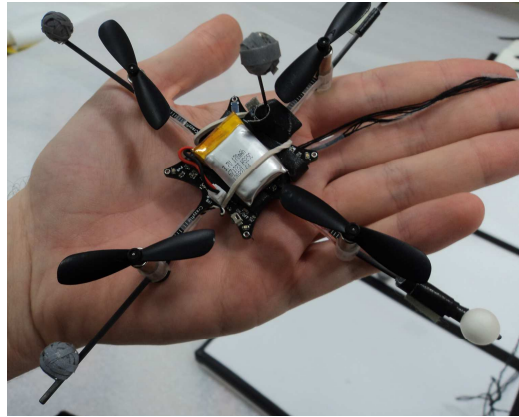
Figure 6.9: Modified Crazyflie with additional carbon fibre sticks in order to attach the markers with a proper distance.
