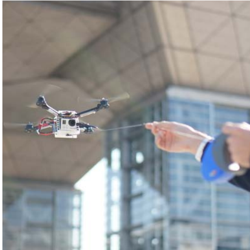
Figure 1.3: Fotokite [14] is a flying camera based on the system designed by Lupashin in [13].
