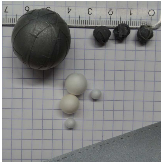
Figure 6.8: Hand made markers. On the left a normal marker used for the MikroKopter quadrotor. On the right the hand made markers with a diameter about 7-8 [mm]. On the bottom of the figure there are the materials used for build the reflecting balls.
