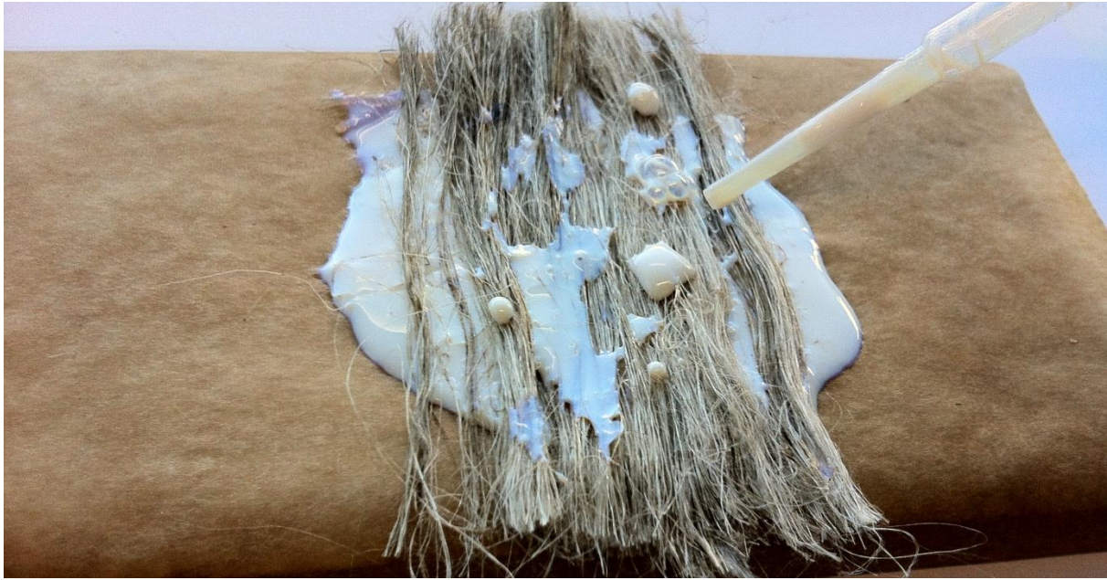
Figure 3.7 Representation of a step during the manufacture of the composite: the spreading of the first thin layer of latex where some flax fibres have been placed on top
