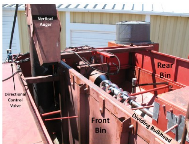
Figura 1: Modifica del cassone per la raccolta selettiva automatizzata (Long D. S., McCallum J. D., Scharf P. A. 2013. Optical-Mechanical System for On-Combine Segregation of Wheat by Grain Protein Concentration, Agronomy Journal • Volume 105, Issue 6 • 2013)
