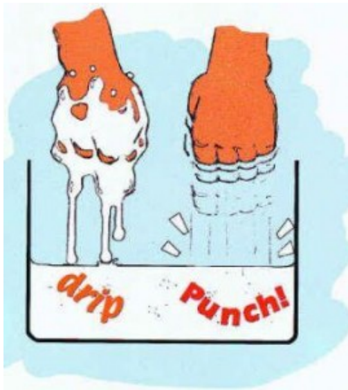
Figure 4.3: Demonstration of oobleck's behaviour depending on the stress applied. Figure for http://junior2m.global2.vic.edu.au .
