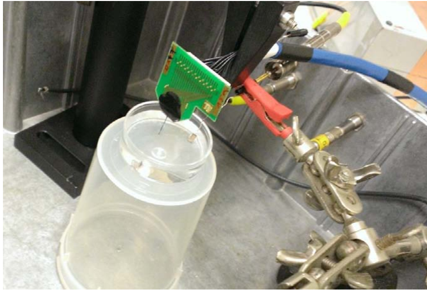
Figure 91: Experiment setup for bias characteristics measurement of a needle chip submersed in electrolyte (PBS solution).
