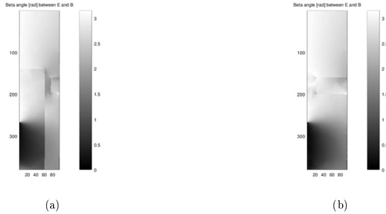
Figure 3.12: Beta angle with (a) and without (b) internal cylinder. Discontinuity of electric field on surface makes Macor ring and Pyrex walls visible.
