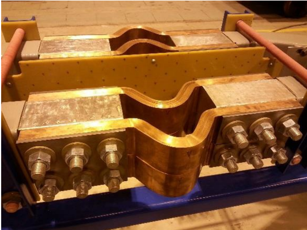
Figure 3.10. Thermal expansion compensators (TEC) [8]
