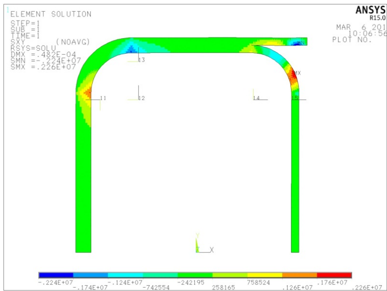
Figure 8.23: Shear xy stress on high voltage insulation and bandage
