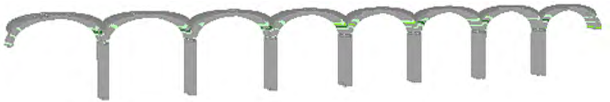
Figure 4.31: deformed shape for the most heavy damage for PGA_1
