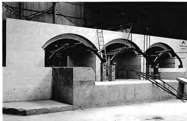
Figure 3.12: Bolton Institute experimental model, case with detached spandrel walls from arches (Professor C. Melbourne, et al., 1997)
