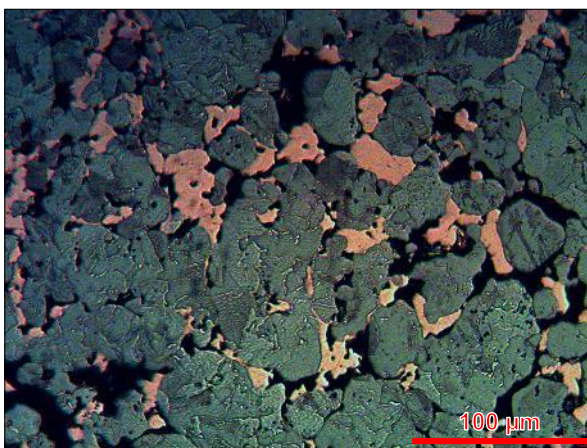
Figura 6.13f. Fersint 180/2.6 - T = 1020 \text{ °C} - HV = 175
