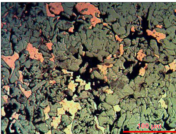
Figura 6.14b. NC 100.24 - T = 1020 \text{ °C} - HV = 104
