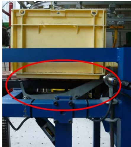
Figure 4.4: The swinging obstruction that controls the access to an elevator.
