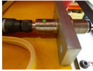
Figure 2.7: A photocell of the double level conveyor belt.
