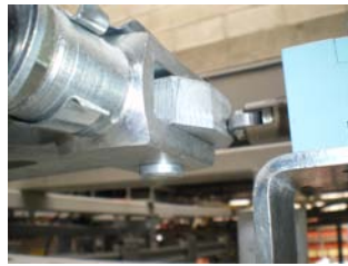
Figure 2.8: A limit switch of the power & free conveyor.
