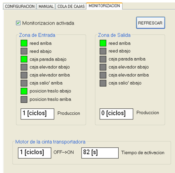
Figure 4.16: Monitoring tab of the HMI for the conveyor belt.
