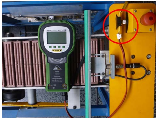
Figure 2.10: The MetraTest AS-i System tester connected to a slave.
