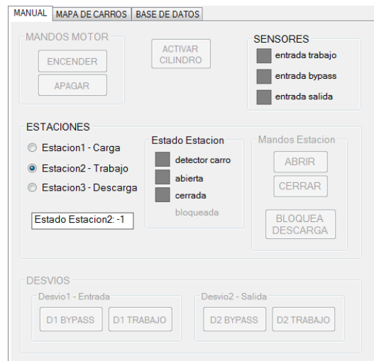
Figure 3.14: Manual tab of the HMI for the power & free conveyor.
