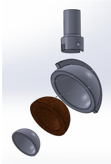
Fig. 6.2) Cup-hosting bowl. Exploded view.
