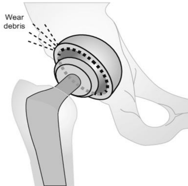
Fig. 2.10) Hip prosthesis biocompatibility and wear debris
