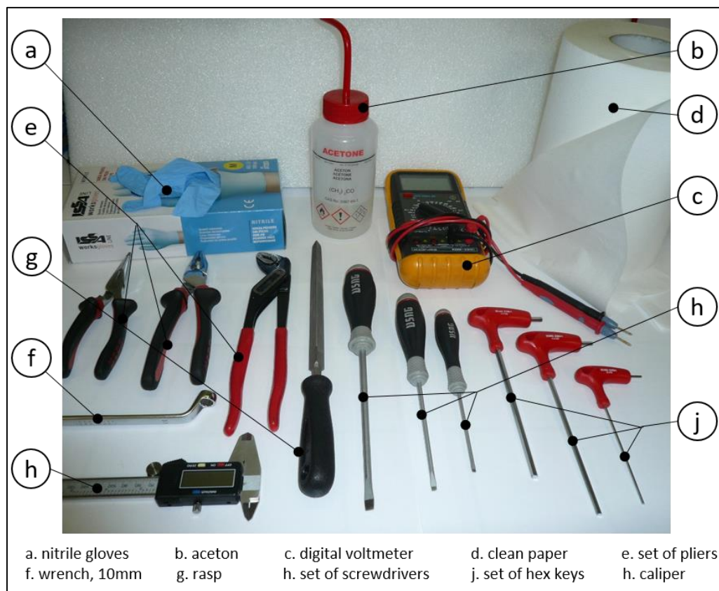
Fig. C.1 Equipment required for the SPES SIS assembly.
