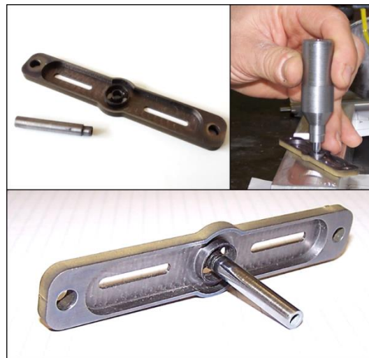
Fig. C.6 Plastic deformation coupling phases.
