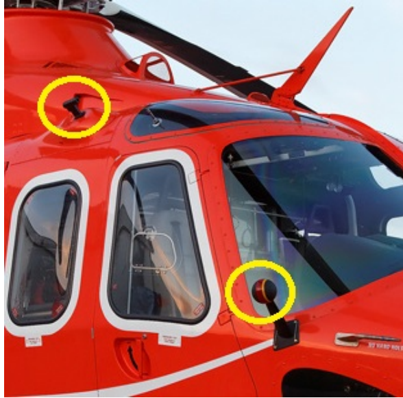
Figure 1.4: Top left: Ice detector, used to detect the presence of liquid water in the air. Bottom right: SLD marker, provides visual information on particle size; if ice grows in the red or yellow area particle size is above certification limits, and flight is not permitted.
