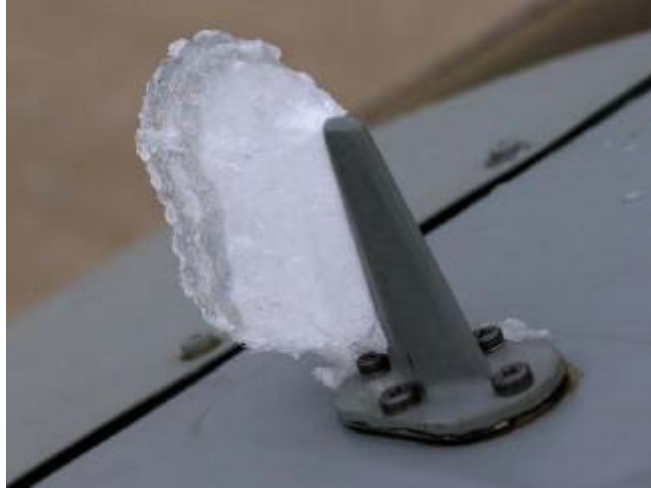
Figure 1.3: Icing on an external probe.
