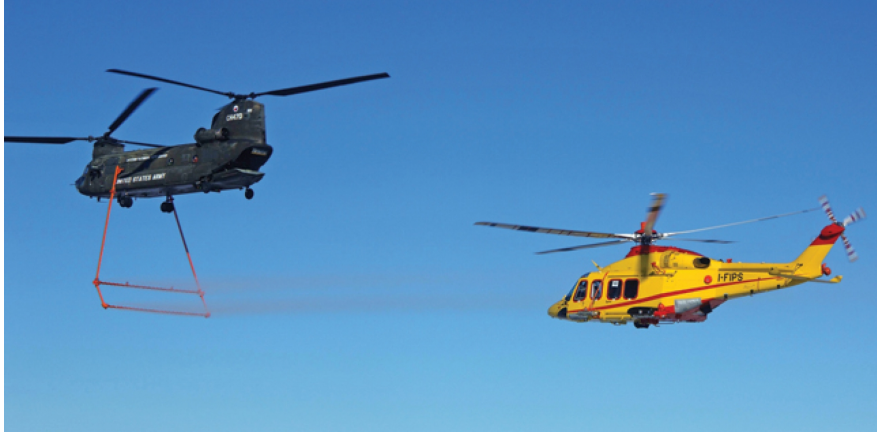
Figure 1.5: AW139 during icing trials; a CH-47 sprays liquid water which reproduce icing conditions, while the tested helicopter follows.
