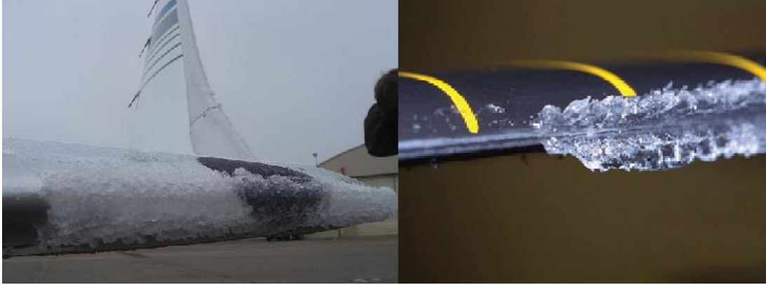
Figure 1.1: Rime ice accretion, left, and glaze ice, right.
