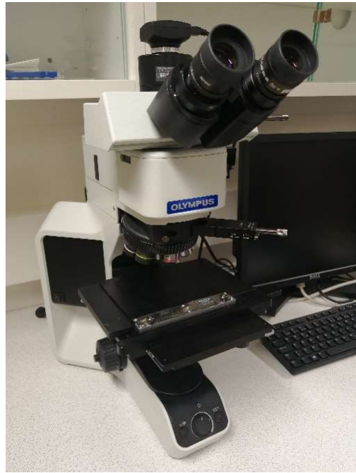
Figure 4.11: OLYMPUS optical microscope used for microstructure examinations
