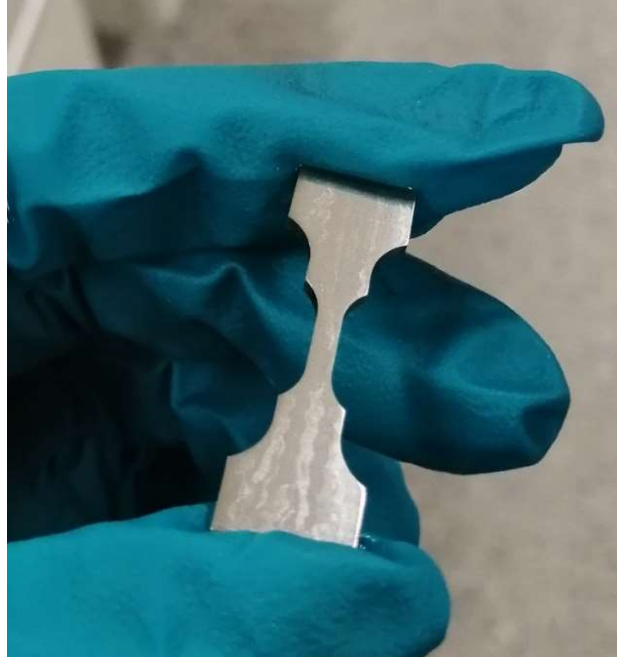
Figure 4.4: DED specimen after O-PS polishing step; Some prior grains are visible to the naked eye
