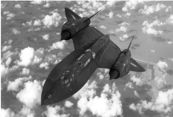
Figure 1.17: SR71 aircraft: first use of beta alloys in aerospace structures. (Courtesy of Lockheed California Co) [9]
