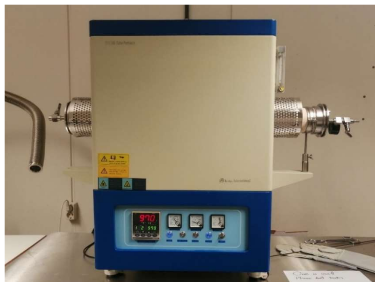
Figure 4.7: Tube furnace used to heat treat the specimens
