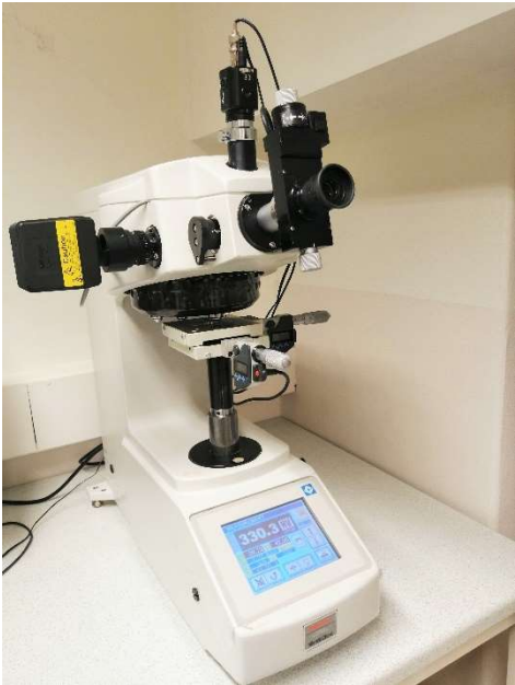
Figure 4.13: Mitutoyo Microwizard Vickers microhardness tester
