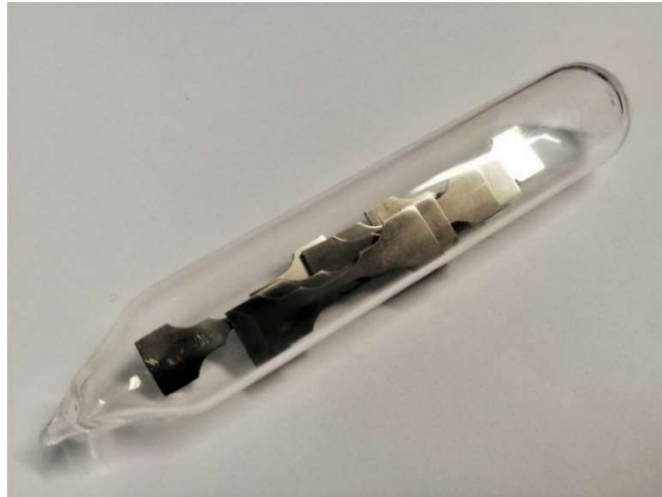
Figure 4.8: Specimens encapsulated in a vacuum glass case to avoid them from oxide formation during their heat treatment
