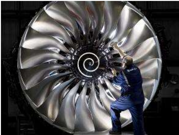
Figure 1.16: The large front fan blades in modern jet engines are now often made from titanium alloys[13]
