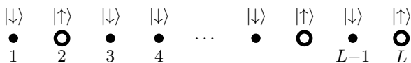
Figure 2.1: Schematical representation of the ultra-cold Rydberg atoms chain. We denote with small filled circles ( \bullet ) the ground states, and with big void circles ( \circ ) the highly-excited Rydberg state.
