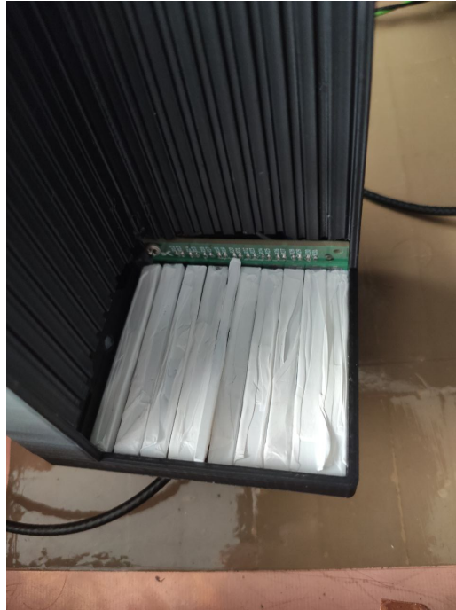
Figure 4.15: Setup for characterizing the position resolving power, using 9 bars.
