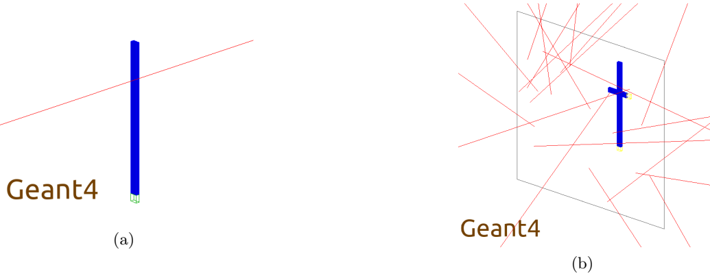
Figure 21: (a) Rendering of the simulation v1 geometry: a muon pencil beam (red) incident on a single scintillator; (b) Rendering of the simulation v2 geometry: muons are generated from a surface (grey), two perpendicular scintillators are present.
