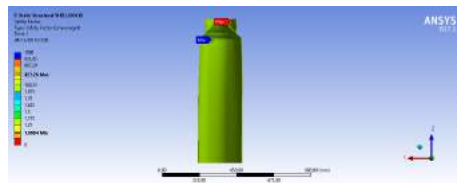
(f) Safety factor, tube overlap.
