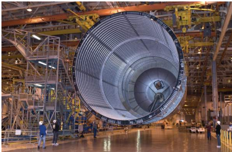
Figure 1.17: The use of aluminum-lithium Al 2195 in manufacturing major External Tank components allowed NASA to reduce the overall weight of the External Tank by 3402 kg
