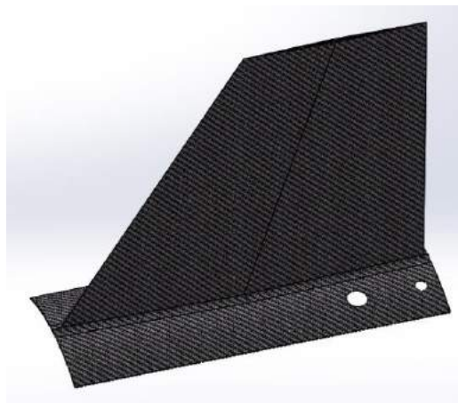
Figure 2.7: Fin and attachment to rocket
