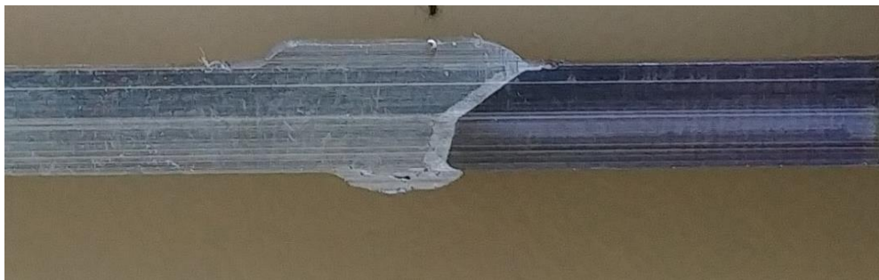
Figure 2.14. HYB dissimilar, trasversal view of a specimen. Aluminium on left side, steel on the right side.
