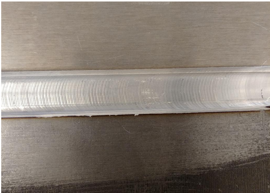
Figure 3.3 Filler material detail
