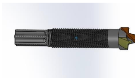
Figure 1.5 Conical pin used for HYB butt joining of plates; (Ø.Grong, Personal Communication)
