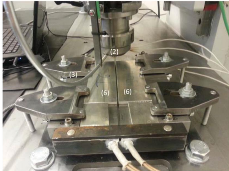
Figure 2.9. Experimental setup of Al-Al HYB configuration: HYB spindle extruder (2), steel fixture (3), aluminium plates to be welded (6).
