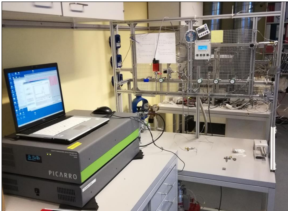
Figure 4. 1 Laboratory station: Picarro analyzer on the left and the extraction line on the background
