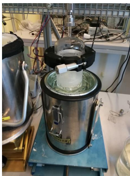
Figure 6. 6 Ethanol-dry ice bath under the glass vessel
