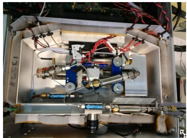
Figure 3. 9 High finesse optical cavity
