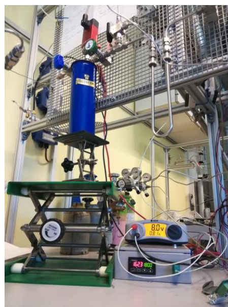
Figure 4. 8 Whole view of the heating system mounted around the sample trap. The blue container helps to keep the heat and accelerate the temperature increasing.
