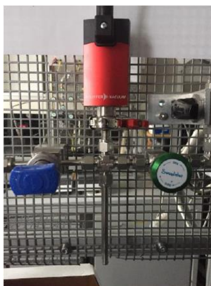
Figure 4. 6 Sample trap between valve 3 (on the right) and valve 4 (on the left)
