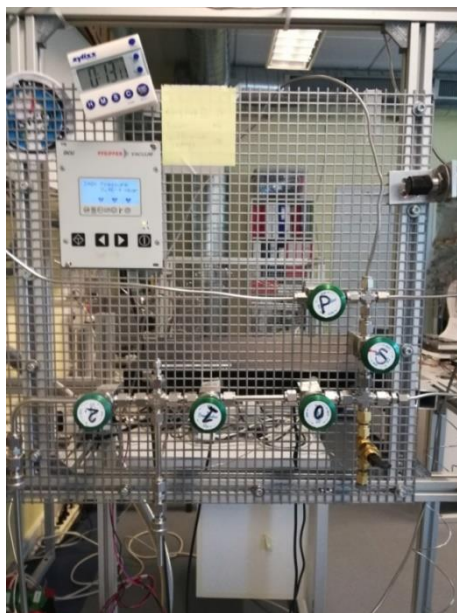
Figure 4. 4 The latest configuration of the extraction line with additional valves: S and P
