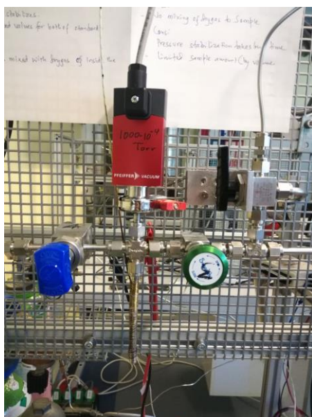
Figure 4. 7 Sample tramp with the high resistance wire wrapped around the tube
