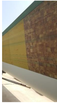
Figure 7.3: The border between the two kinds of wood that compose the blade cover.
