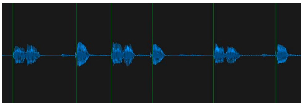
Figure 4.2: Example of false negative. Two consecutive notes, in which the audio signal is not clearly separated, are captured as one single onset by the transformation function of Sonic Visualizer.
