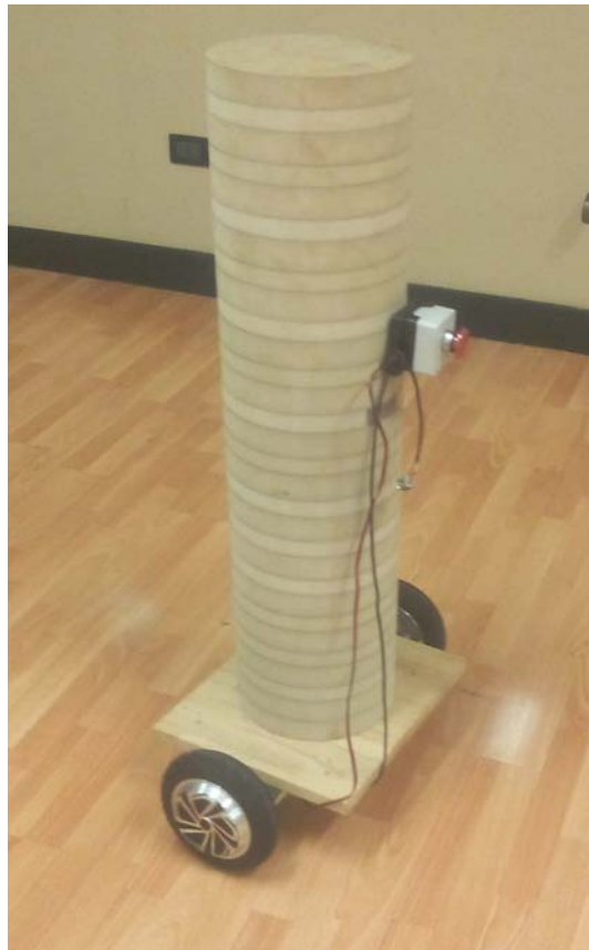
Figure 77: Wood cylinder anchored to the self-balancing transporter. The simple and regular geometry and the knowledge of weight and dimensions, makes it easy to model it into the simulator.
