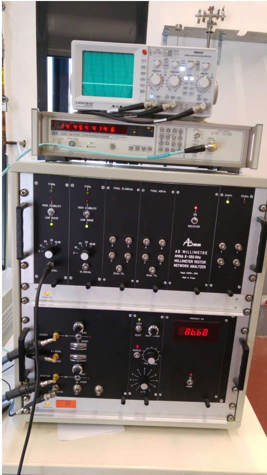
(a) The MVCA apparatus, with an oscilloscope to control the signal.
