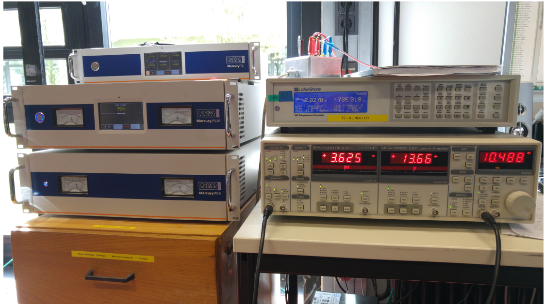
Figure 4.3: The iPS, iTC and Lakeshore for temperature and magnetic field control
