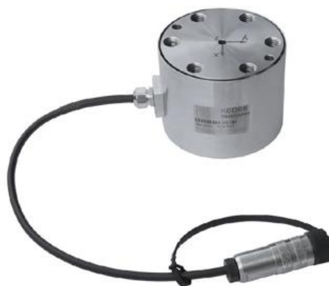
Figure 2.3.2.1: The 6-axes load cell that was used
