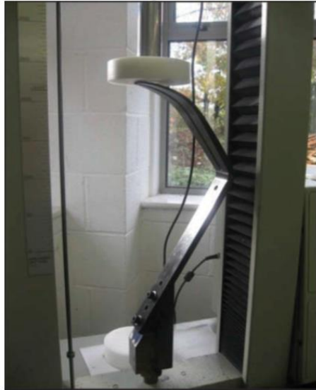
Figure 1.3.2.1: Testing machine and ESRP prosthesis (upside down)
