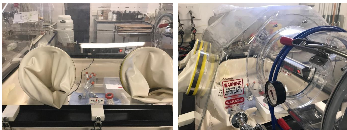
Fig. 5.7: Glovebox under nitrogen to prepare DPPH solution and to preserve the cuvettes
