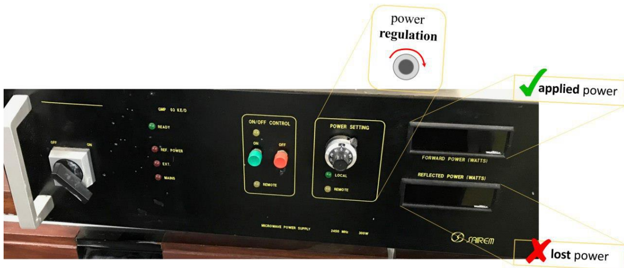
Fig. 2.2: Microwave power supply to regulate the power
