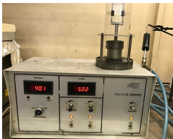
Fig. 4.6: Laboratory equipment for LOI test
