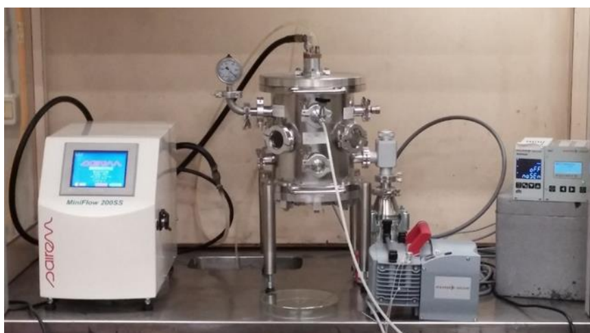
Fig. 5.12: Microwave Miniflow 200SS Plasma Equipment
