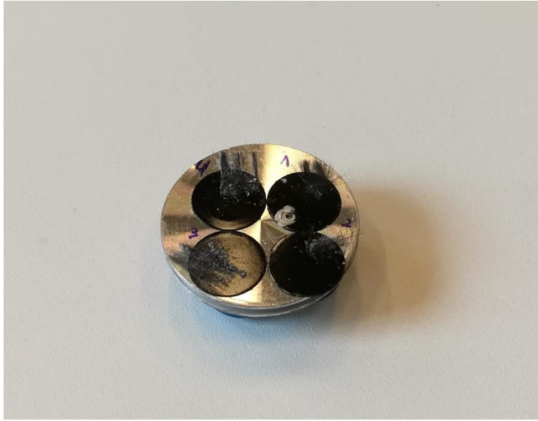
Fig. 3-4: surface treated C fibers prepared for SEM analysis.
