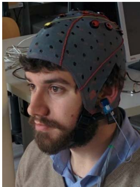
Figure 3 Non-invasive EEG electrode headset
