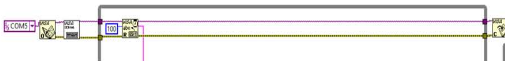
Figure A.11. The serial communication is set on the COM5 USB port where the Arduino-based hardware is connected to the PC.
