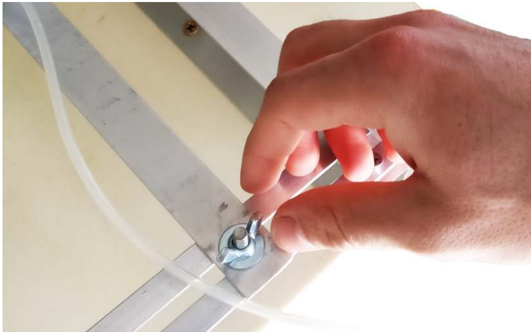
Figure 5.5. The mobile bar of the bench may be fixed on the guides by means of a wingnut.
