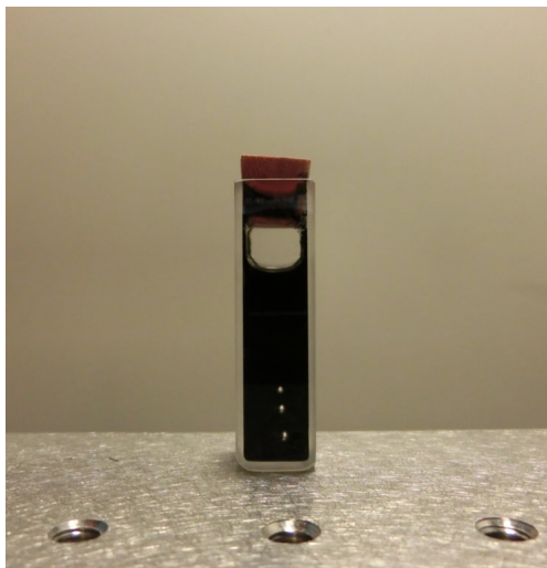
Figure 4.1.4: Image of the cuvette containing the SWCNT aqueous dispersion employed in the fluorescence emission measurements.
