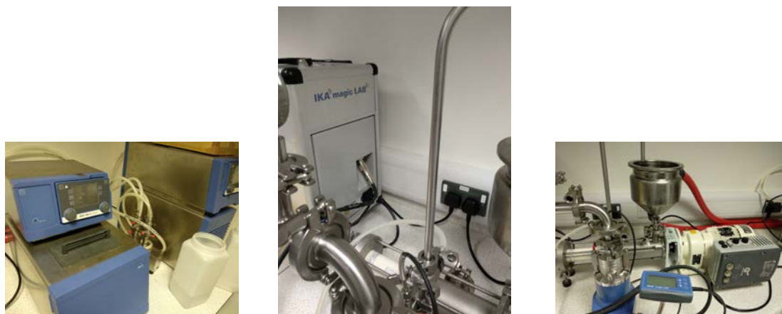
Figure 2.6: IKA Magic lab a) cooling and heating baths b) box for transportation c) main part of the equipment
