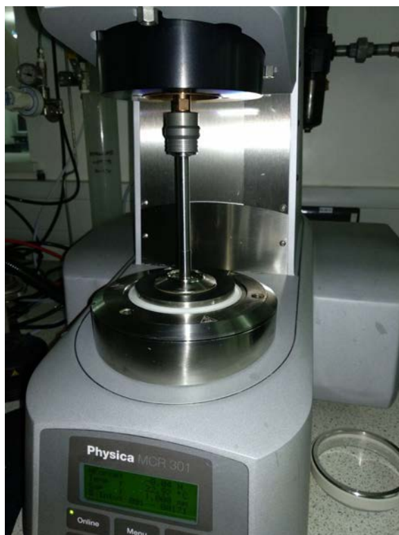
Figure 2.11: Rheometer used for the experiments
