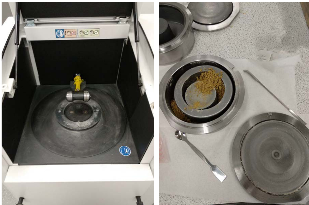
Figure 2.10: a. Milling machine. b. cylinders containing the sample
