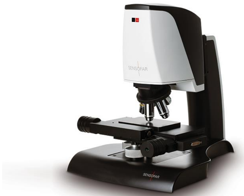
Figure 2.4 Sensofar® S Neox optical profiler used in T.E.S.I. laboratory in Rovigo; adapted from [20].
