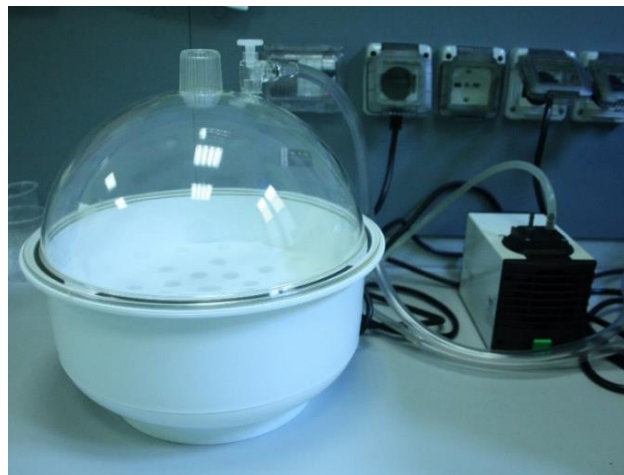
Figure 2.6 Desiccator connected to the vacuum pump used in the BIAMET laboratory.
