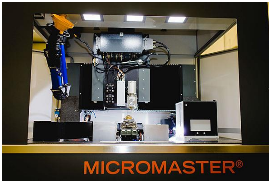
Figure 2.2 Kugler MICROMASTER ® 5X micromiller used in T.E.S.I. laboratory in Rovigo; adapted from [19].
