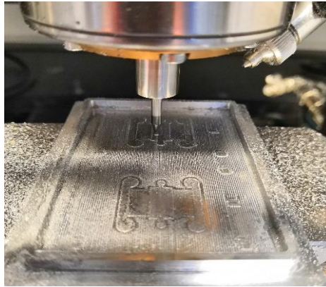
Figure 2.3 The milling of the microfluidic platform mold.
