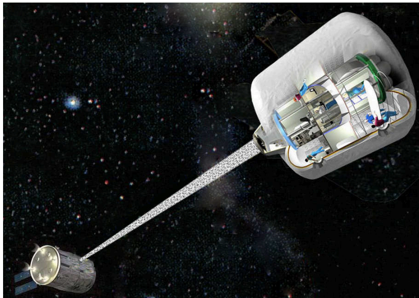
Figure 3.4. Concept art of a tethered spinning spacecraft for the generation of artificial gravity (Landsdorp et al. [5])
