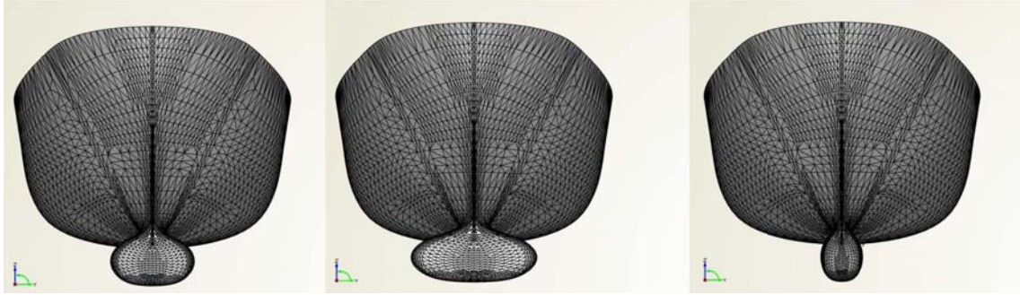
Figure 5.4: Bulb's width: from left to right the baseline, the upper bound and the lower bound configurations.
